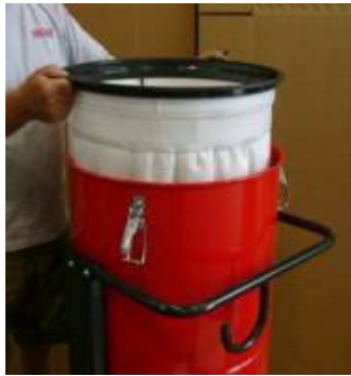
Dust collector filter
